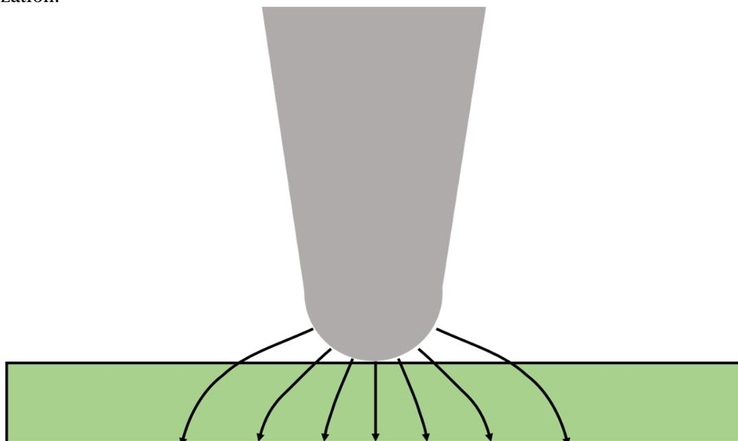
**Fig. S12: Schematic of *in situ* application of electric fields in DF-TEM.** Schematic of electric field applied through a tip. Demonstrates mixture of in-plane and out-of-plane fields.
