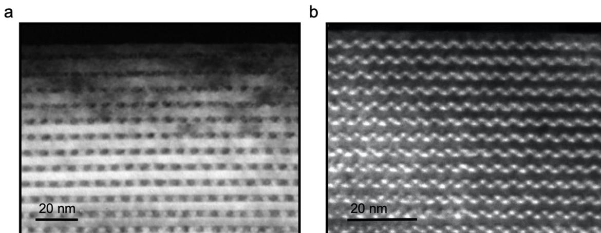
**Fig. S11: DF-TEM Analysis.** (A) DF-TEM image taken using the  $[220]_o$  reflection, giving rise to contrast from domains with opposing displacement along the  $c$ -axis. (B) DF-TEM image taken using  $[008]_o$  reflection, giving rise to contrast from domains with opposing displacement along the  $a$ -axis
