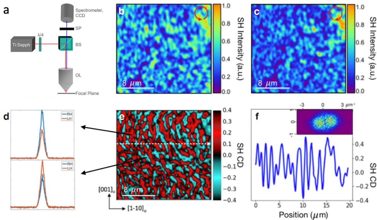
**Fig. S4: Experimental Details of SHG-CD.** (A) Experimental layout for the SHG-CD measurements. (B,C) Examples of SHG images acquired with RC/LC excitation. (D) Examples of SHG spectra acquired at a single point in a RC dominant domain (top) and a LC dominant domain (bottom). (E) SHG CD calculated from the images shown in (B) and (C). (F) Line profile along the dotted line shown in (E) and FFT of the SHG CD showing domain elongation along the  $[001]_o$  axis (inset).
