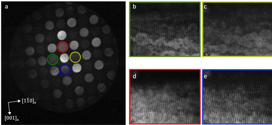
**Fig. S6: Example of 4D-STEM Analysis.** (A) Normalized CBED pattern extracted from entire region in Figure 3a. (B-E) Virtual images that are formed by selected the different diffraction disks along  $[001]_o$  (red/blue) and  $[1\bar{1}0]_o$  (green/yellow) directions.
