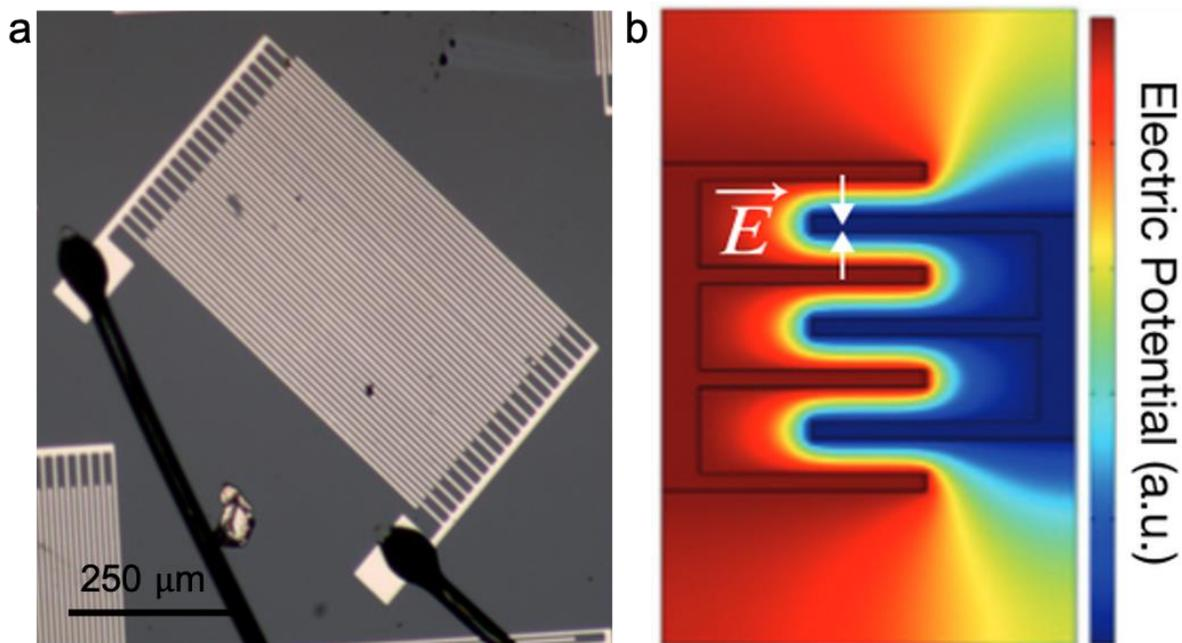
**Fig. S7: Structure of Interdigitated Electrodes.** (A) Image of representative IDE device used. (B) Calculated electric potential for an IDE device, demonstrating opposite electric field across neighboring fingers.
