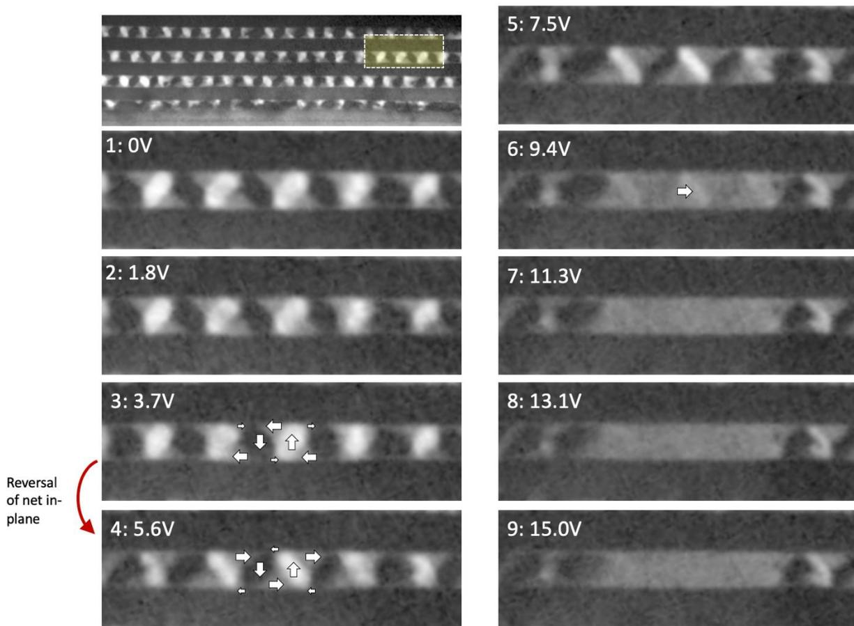
**Fig. S13: DF-TEM imaging of chiral phase transition.** DF-TEM images for increasing applied voltages showing microscopic restructuring across the in-plane reversal of polarization and transition to pure ferroelectric state at higher voltages
