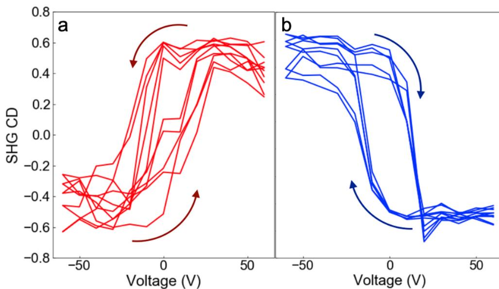
**Fig. S8: SHG-CD Hysteresis.** (A-B) Hysteresis repeated in five different RC and LC oriented chiral domains, respectively, which show the expected mirrored behavior in the CD signal.
