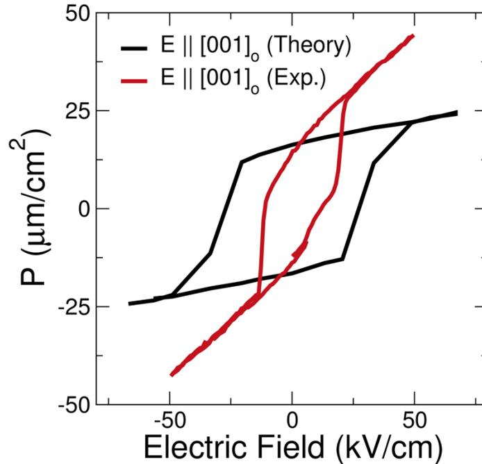
**Fig. S9: Hysteresis Loops.** Raw data for polarization vs. electrical field measurements performed with the electric field along the  $[001]_o$  axis (red). Polarization response from second principles is seen in black.
