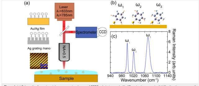
Figure 1: (a) Schematic of experimental arrangement and range of SERS substrates used with different enhancements. (b) Vibrational resonances of benzenethiol with nuclear motion as indicated and (c) corresponding SERS spectrum on a Ag nanosubstrate.
