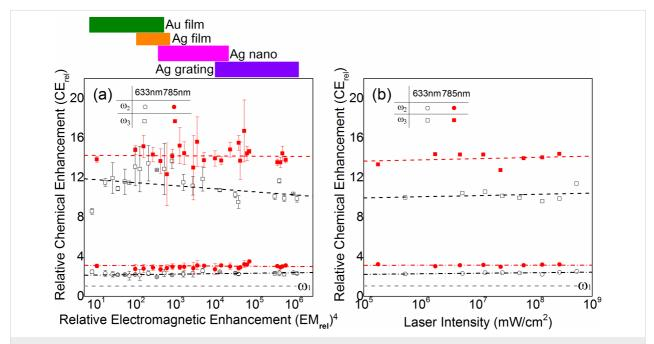
**Figure 3:** (a) Relative Chemical enhancement (CE<sub>rel</sub>) factor versus relative electromagnetic enhancement (EM<sub>rel</sub>) for different substrates with 633 nm (black) and 785 nm (red) excitation (with incident laser power of  $2 \times 10^7$  mW/cm<sup>2</sup>)  $\omega_2$  and  $\omega_3$ . (b) Chemical enhancement as a function of incident laser intensity for the Ag nanosubstrate with 633 nm (black) and 785 nm (red) excitation.
