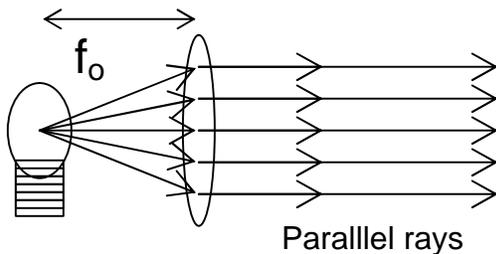
The point source is the object and the object distance  $d_o$  is the focal length  $f$ . With  $d_o = f$ , equation (1) predicts that  $d_i = \infty$ . The rays from the lens converge "at infinity".
