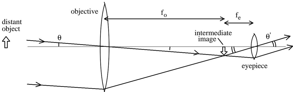
Notice that the distance between the two lenses is  $\ell = f_o + f_e$ . From the diagram above, one can show that the angular magnification can also be written as  $M = \frac{f_o}{f_e}$ , the ratio of the focal lengths of the objective and eyepiece lenses.
