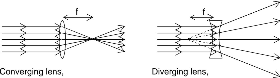
A converging lens can be used to form an image on a screen of an object. *The lens equation* relates the focal length  $f$  of a lens, the object distance  $d_o$  and the image distance  $d_i$ ,
