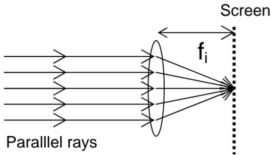
To do this in the experiment you will first need to produce the parallel beam of light with which to measure the focal distances of your telescope lenses. This will be produced by the complementary method where a (different) lens is used to convert a point source of light (the filament at the center of the light bulb) into a parallel beam of light, as shown below.
