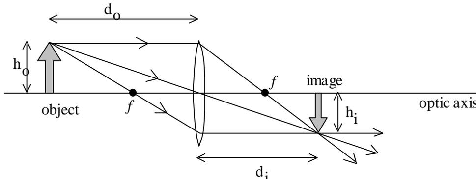
In the diagram above, the points labeled  $f$  are the focal points of the lens. *The lateral magnification*,  $m$ , of the image is defined as  $m = \left| \frac{h_i}{h_o} \right|$ . From the diagram above, one can show that  $m$  can also be written as:  $m = \left| \frac{d_i}{d_o} \right|$ .
