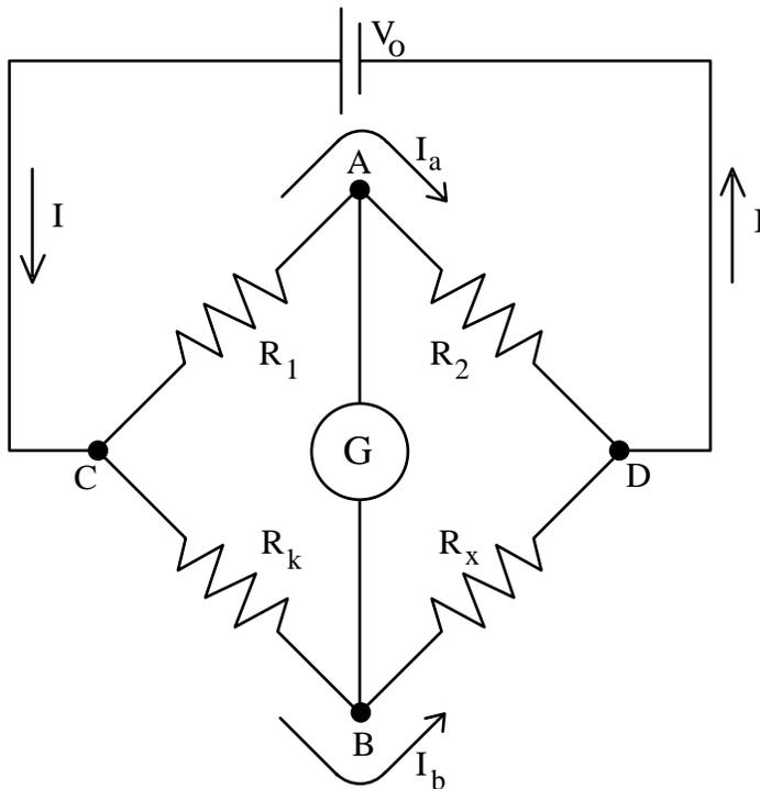
The unknown resistor is  $R_x$ , the resistor  $R_k$  is known, and the two resistors  $R_1$  and  $R_2$  have a known ratio  $R_2/R_1$ , although their individual values may not be known. A galvanometer  $G$  measures the voltage difference  $V_{AB}$  between points  $A$  and  $B$ . Either the known resistor  $R_k$  or the ratio  $R_2/R_1$  is adjusted until the voltage difference  $V_{AB}$  is zero and no current flows through  $G$ . When  $V_{AB} = 0$ , the bridge is said to be “balanced”.
