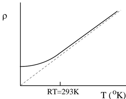
At  $T = 20\text{C}$ , the resistivity of pure, defect-free, copper is  $\rho_{RT} = 1.678 \times 10^{-8} \Omega \cdot \text{m}$ . (RT stands for room temperature.)
